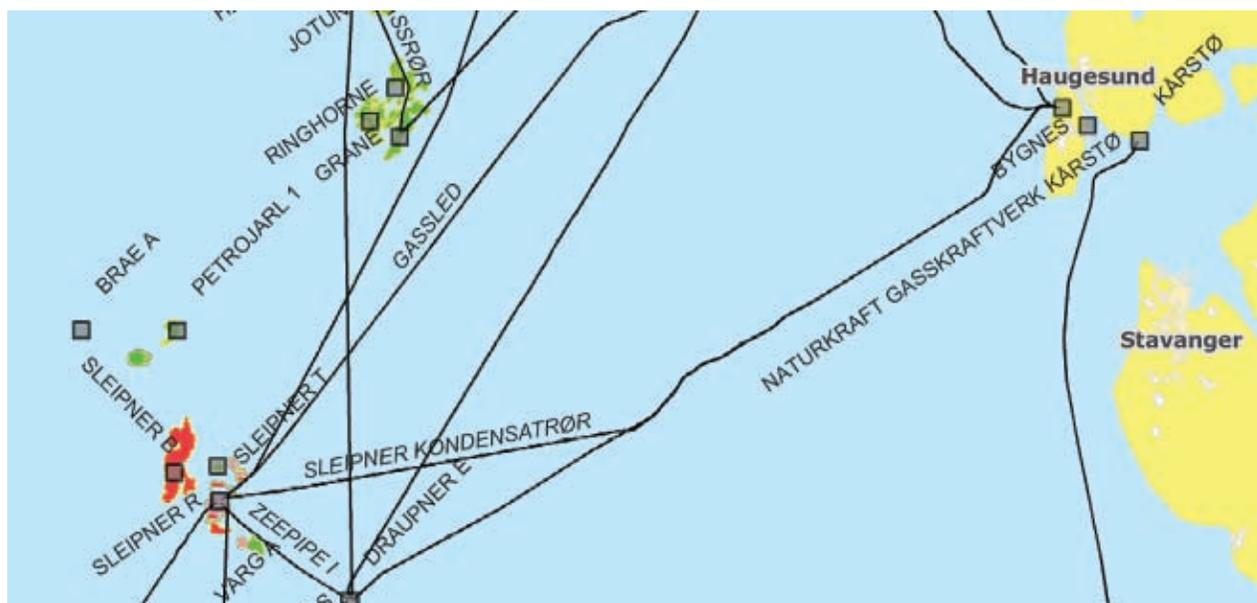
The Sleipner East condensate pipeline runs from Sleipner A to Kårstø. Map: Norwegian Petroleum Directorate
