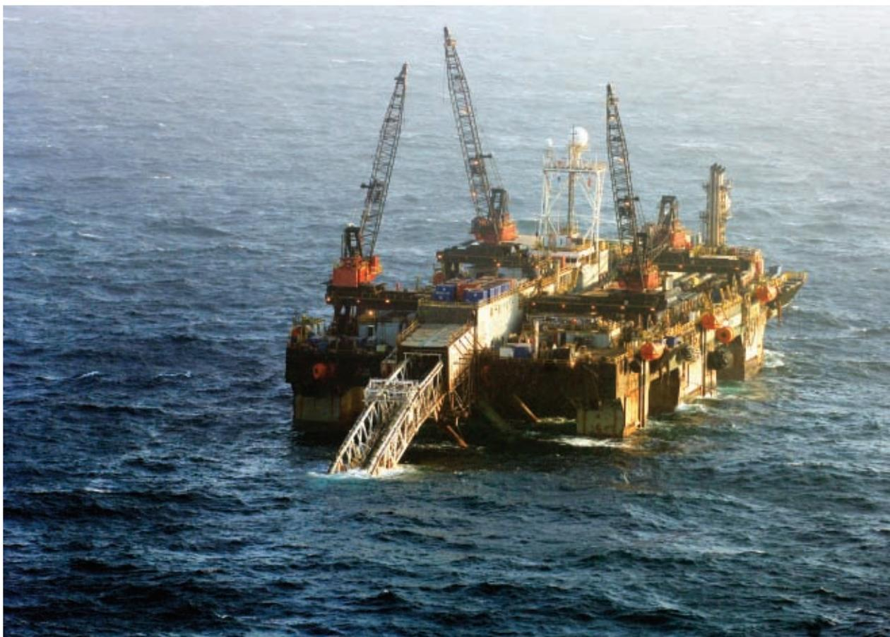
*The Acergy Piper pipeline laybarge. Photo: Marit Hommedal/Statoil*
