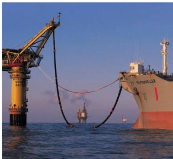
*The Gullfaks B loading buoy with the Polytraveller shuttle tanker. Photo: Øyvind Hagen/Statoil*
